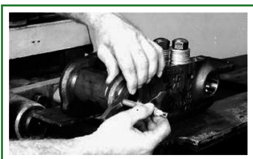
T96275-UN: Bushing Projection Measurement
