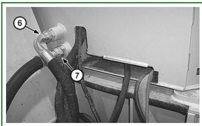
T200325A-UN: Hydrostatic Reservoir Plumbing
