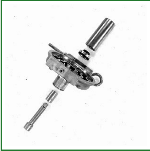
RW21162-UN: Installing A New Lip Seal With A Socket
