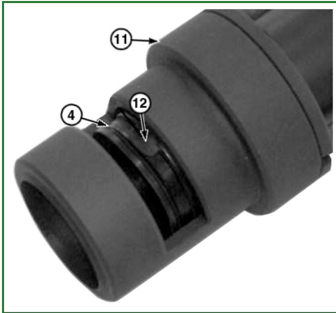
TX1060099A-UN: JDG10583 Seal Installation Tool
