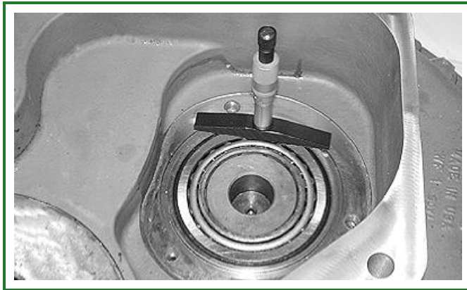
T199781A-UN: Second Idler Pinion Gear Shaft End Play Measurement
