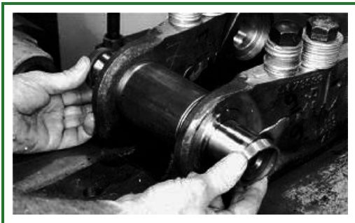
T96278-UN: Thrust Ring Installation
