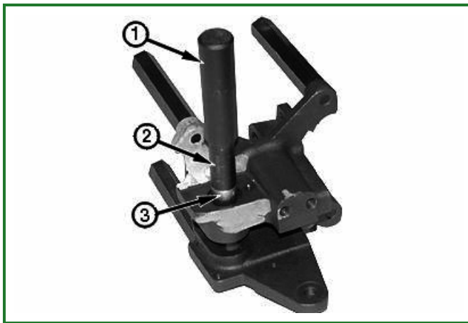
T121385B-UN: Install Detent Shaft Bearing
