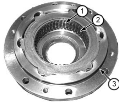
1— Friction Disk (7 used) 3— O-Ring 2— Separator Plate (8 used)
